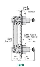
(Max. fluid level of the hydraulic reservoir above the banjo bolts)
