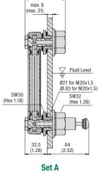
(Max. fluid level of the hydraulic reservoir between the banjo bolts)
