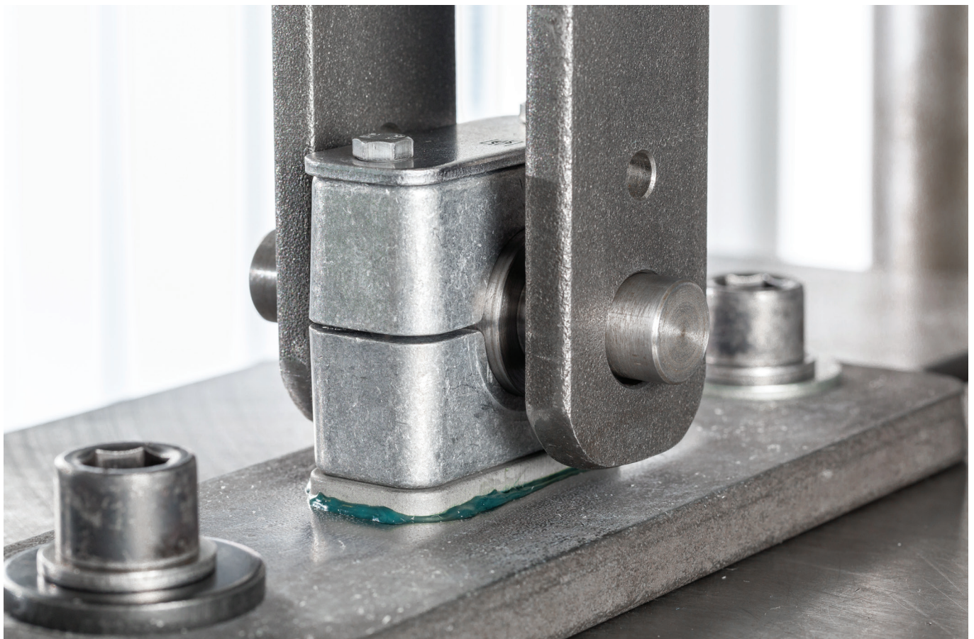
Tensile testing of the STAUFF Bond Plate (type SBP) with STAUFF Bond Adhesive (type CB420-50E) in the STAUFF Technology Centre. Please contact STAUFF for detailed test reports.
